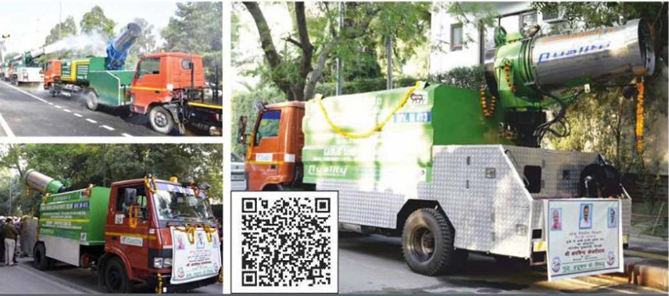
The anti-smog gun is fed by a 5,000-litre water tank and can work for 3-4 hours continuously.
