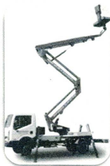
Sky Lift / Hydraulic Aerial Access Platform:
